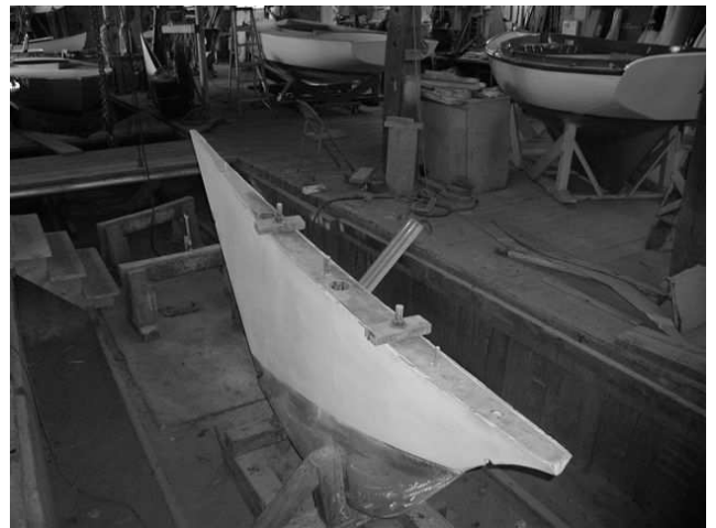
A-144 keel in line for attachment
