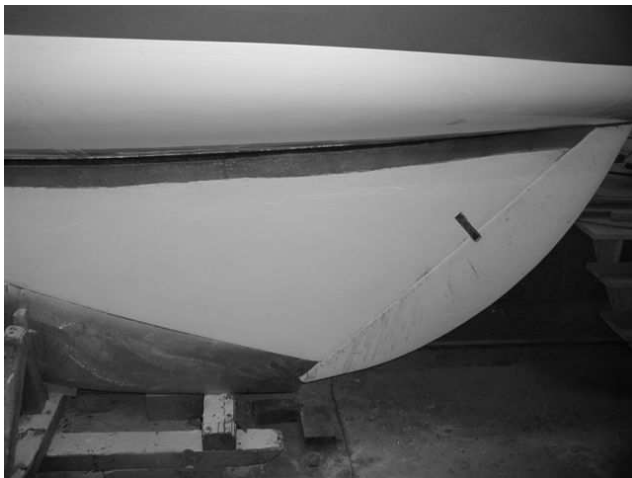
Extra care to prevent keel crack
